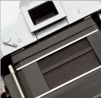
Above: Vertical running focal-plane shutter made with cloth blinds.
